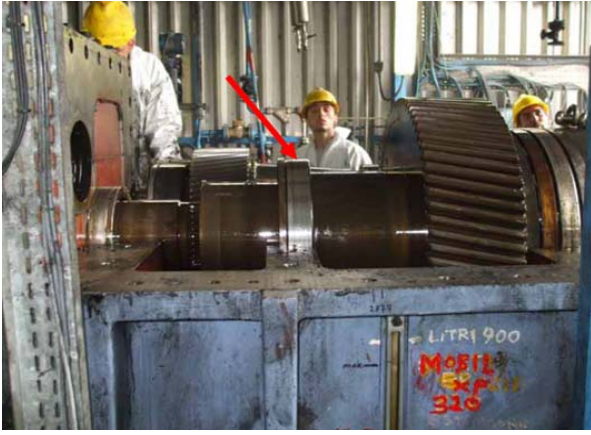
Fig. 3 - Crankcase after removal of top cover;
