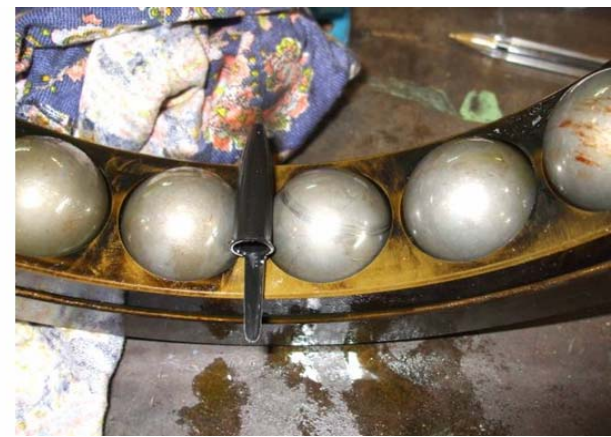
Fig. 6 - 151 Bearing with circular wear signs;
