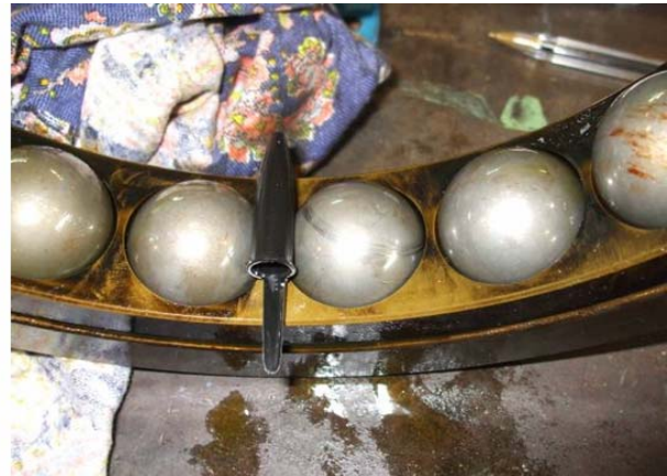
Fig. 5 - 151 Bearing with circular wear signs;
