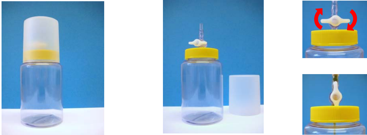
Figure 3: Main structural features of the UCVD.
