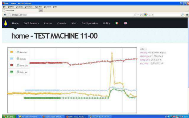
Figure 4: Monitoil-Software – Web page. The increase of yellow line indicate the induced contamination of a different fluid in the system (ester in a mineral oil).
