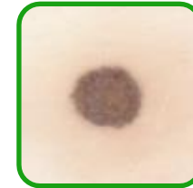
Severely oxidized oil - dark center (sludge) with distinct outer ring
