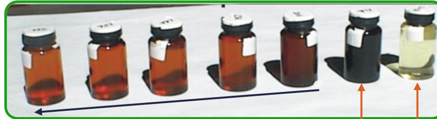
Progressive removal of oxide insolubles
